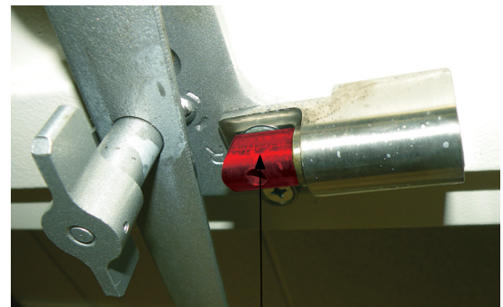
Stop Shown Before Door is Fully Opened
